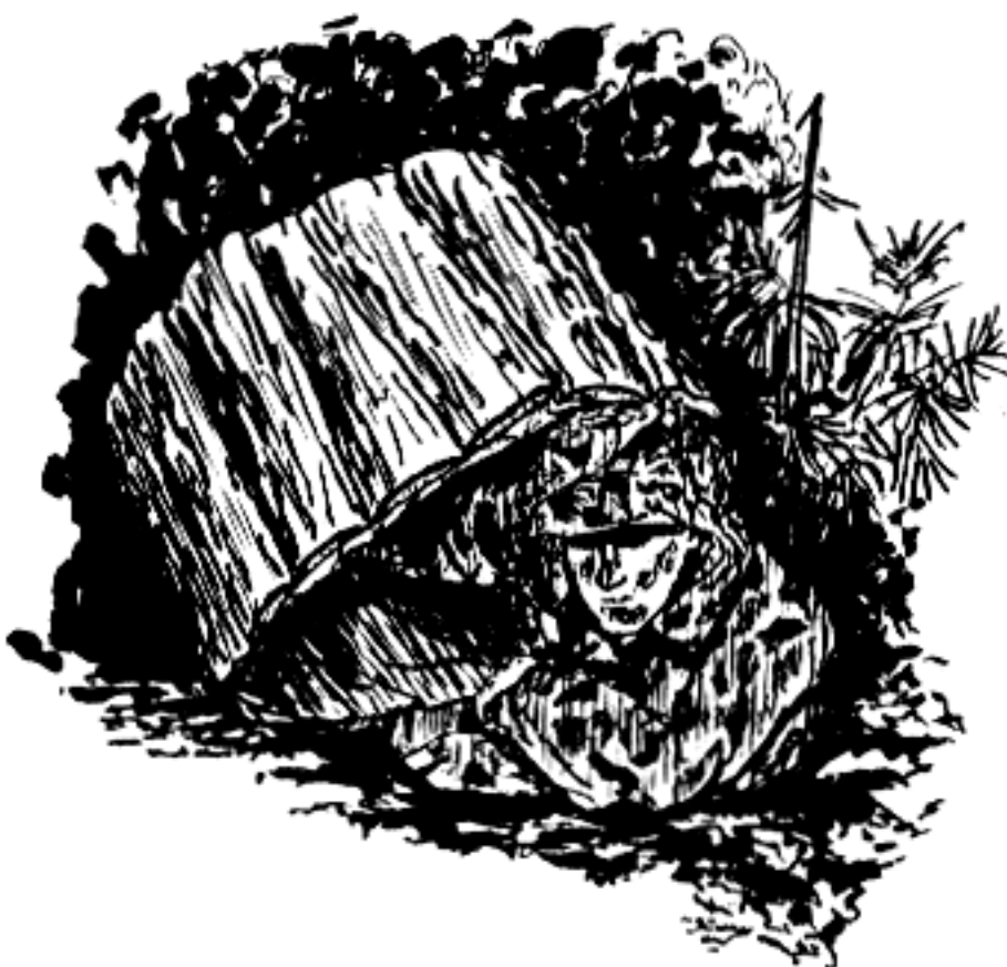
Figure 26. Cover made from burlap and tree bark.
